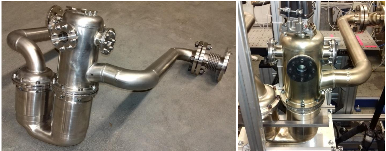
Figure 5: Optically accessible ammonia generator ready for installation (left) and installed at the test rig (right)
