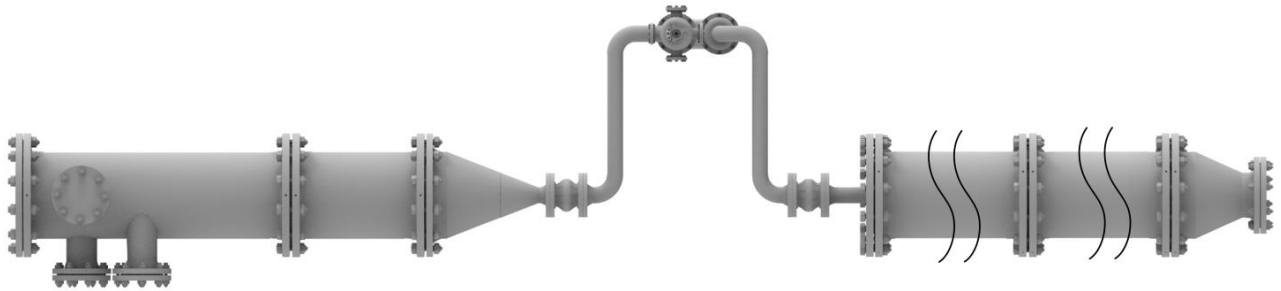
Figure 4: Setup of ammonia generator at hot gas test rig
